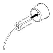
Connect the AM loop antenna to the AM jack on the back of the main unit. Adjust the position of the antenna for optimal reception.
