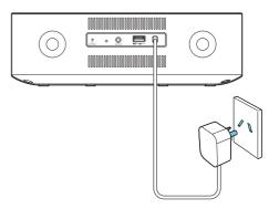
Connect the AC power cord to the wall outlet.
