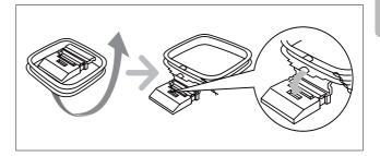
2 Connect the MW loop antenna to the MW AERIAL jack on the rear of the main unit.
