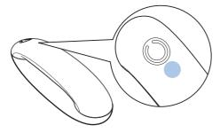
Charge your handset by docking it in either direction. When the handset is placed correctly on the base station, you hear a docking tone (see 'Set the docking tone' on page 22).
