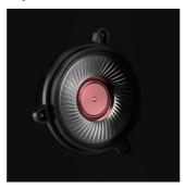
Layered Motion Control (LMC) drivers feature a multi-layered polymer diaphragm that encases a layer of damping gel. These layers form a flexible boundary and – together with the gel – absorb and dampen any exaggerated frequencies, resulting in a smooth and flatter frequency response. The result is a more balanced, natural and refined range of high-frequency sounds.
