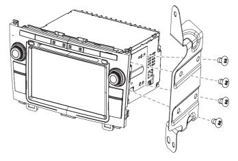
4 Fix the unit to the dashboard with screws (supplied by the car manufacturer).
