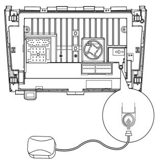
2 Stick the other end of the GPS antenna to a surface for signal reception.
