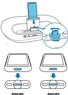
**3** Adjust the bumpers on both sides of the connector to stabilize the phone.
