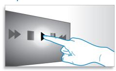
Touch controls allow you to control the volume as well as other playback options by simply pressing the touch sensitive controls on the main unit.
