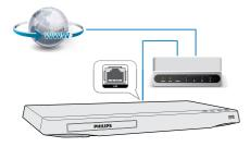
For Wi-Fi, connect a Philips Wi-Fi USB adapter (named WUB1110) to the • (USB) connector on the front panel of this player.
