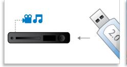
The Universal Serial Bus or USB is a protocol standard that is conveniently used to link PCs, peripherals and consumer electronic equipment. Hi-Speed USB devices have a data transfer rate of up to 480 Mbps - up from the 12 Mbps of original USB devices. With Hi-Speed USB 2.0 Link, all you have to do is plug in your USB device, select the movie, music or photo and play away.
