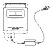
3 Connect the other end of the AC adaptor to the wall outlet.
