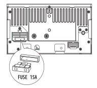
If the fuse gets damaged immediately after it has been replaced, there may be an internal malfunction. In such case, consult your Philips dealer.
