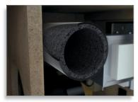
Philips Sound Purification Duct (SPD) bass port technology delivers the deep, pure tones of the original bass sound. Using an SPD foam material to process the inner surface of the bass pipe, the special acoustic damping invented by Philips reduces noise turbulence and stabilizes the tuning frequency. Philips technical and consumer tests confirm this buffer provides less colored, purer quality bass.
