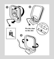
Position the antenna as far as possible from a TV, VCR or other radiation source.
