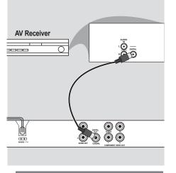
Receiver has a PCM, Dolby Digital or MPEG decoder
