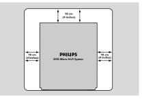
The ventilation should not be impeded by covering the ventilation openings with items, such as newspapers table-cloths, curtains, etc.
