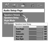
4 Use ◀ ► keys to set the volume level for each speaker (-6dB ~ +6dB) and press OK to confirm. 5 Use ▲▼ keys to highlight { Speakers Delay }, then press ▶.
