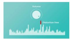
Anti-Clipping lets you play music louder and keeps the quality high, even when the battery is low. It accepts a range of input signals from 300 mV to 1000 mV and keeps your speakers safe from damage by distortion. This built-in function monitors the musical signal as it goes through the amplifier and keeps peaks within the amplifier's range, preventing the audio distortion caused by clipping without affecting loudness. A portable speaker's ability to reproduce musical peaks decreases along with
