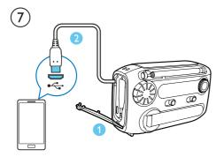
3 Slide the power source selector to CHARGE MOBILE. (Fig. ® )
