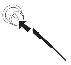
1 Connect the supplied FM antenna to the FM AERIAL socket on the unit.
