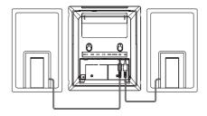
1 Connect the two front speaker cables to the SPEAKERS terminals: right speaker to "RIGHT" and left speaker to "LEFT".
