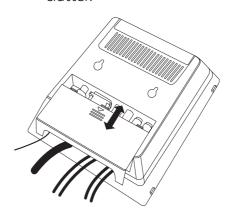
2 Align the side marked PRESS▼ of the stand to the slots at the bottom of the set.
