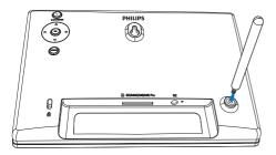
2 Screw the stand into the stand hole firmly.
