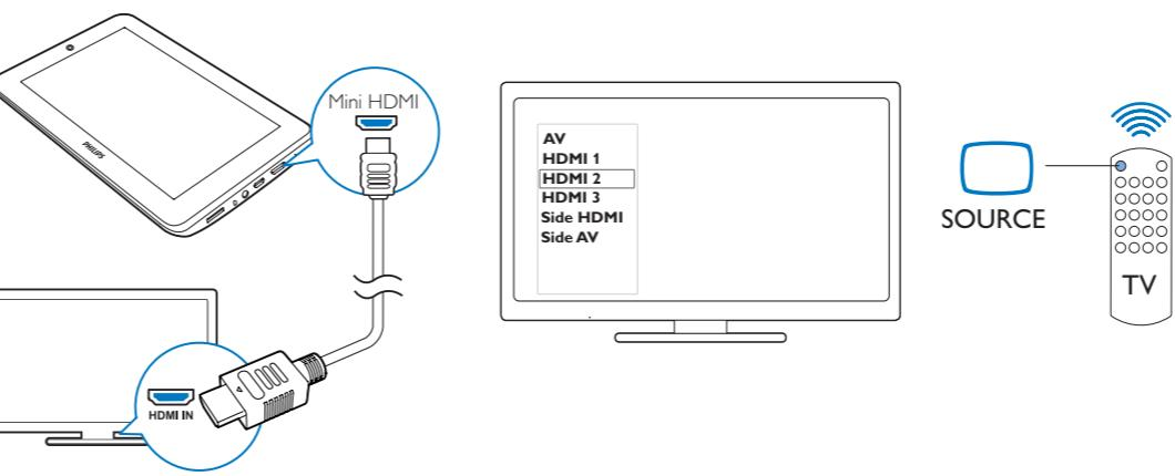
EN Through Mini HDMI cable connect PI3110 to an HDTV. On the remote control, press the source button to select the Mini HDMI input connector.
