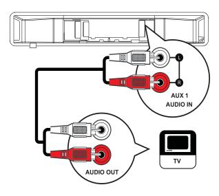
1 Connect the audio cables (not supplied) to the AUDIO IN-AUX1 jacks on the Home Theater System and the AUDIO output jacks on the TV.
