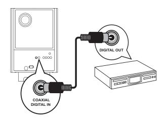
1 Connect a coaxial cable (not supplied) to the COAXIAL DIGITAL-IN jack on the subwoofer and the COAXIAL/DIGITAL output jack on the device.
