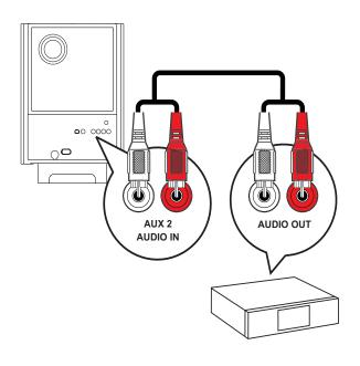
1 Connect the audio cables (not supplied) to the AUDIO IN-AUX2 or AUX3 jacks on the subwoofer and the AUDIO output jacks on the device.
