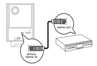
1 Connect an optical cable (not supplied) to the OPTICAL DIGITAL-IN jack on the subwoofer and the OPTICAL/SPDIF output jack on the device.
