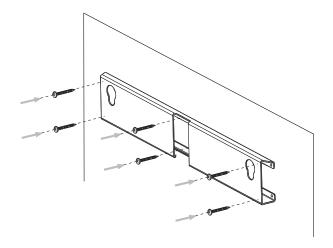
7 Hook this Home Theater System firmly onto the mounted bracket. Slide the knobs through the key holes to lock into position.
