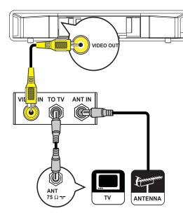
If your TV only has a single Antenna Input jack (labeled as 75 ohm or RF In), use a RF modulator to view the disc play on the TV.
