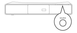
Press SOURCE button repeatedly to select: DISC > RADIO FM > COAXIAL INPUT > OPTICAL INPUT > AUX1 INPUT> AUX2 INPUT > AUX3 INPUT > MP3 LINK > USB > DISC ...
