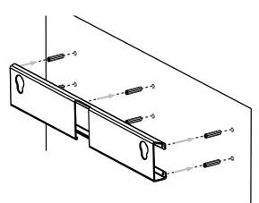
6 Secure the bracket onto the wall with screws (not supplied).
