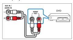
1 Using an analog cable, connect the AUX connectors on your SoundBar to the AUDIO OUT connectors on the TV or other device
