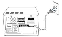
Connect the AC power cord to the wall power socket.
