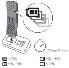
Flashing: low battery Scrolling: charging in progress
