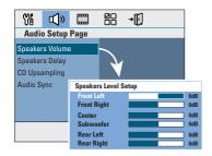
④ Use ◀ ► keys to set the volume level for each speaker (-6dB ~ +6dB) and press OK to confirm. 5 Use ▲▼ keys to highlight { Speakers Delay } and press ▶.
