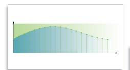
192 kHz sampling enables you to have an accurate representation of the original sound curves. Together with a 24-bit resolution, more information is captured from the original analogue sound wave form, giving a much richer audio reproduction.
