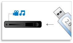
The Universal Serial Bus or USB is a protocol standard that is conveniently used to link PCs, peripherals and consumer electronic equipment. Hi-Speed USB devices have a data transfer rate of up to 480 Mbps - up from the 12 Mbps of original USB devices. With Hi-Speed USB 2.0 Link, all you have to do is plug in your USB device, select the movie, music or photo and play away.
