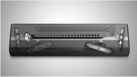
Microbeam technology enables the delivery of powerful, precise sound from a compact form factor. The four high sensitivity drivers (two at the sides and two centered) are arranged in a cross-firing configuration, allowing sound to beam across a 180-degree soundstage with a very wide sweet spot. The effect is a compact, dynamic home cinema speaker that immerses you deeper into the action.
