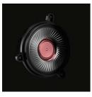
Layered Motion Control (LMC) drivers feature a multi-layered polymer diaphragm that encases a layer of damping gel. These layers form a flexible boundary and – together with the gel – absorb and dampen any exaggerated frequencies, resulting in a smooth and flatter frequency response. The result is a more balanced, natural and refined range of high-frequency sounds.
