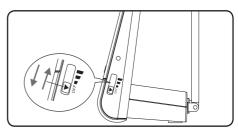
**3** Turn the TV or FM radio to the desired channel/station. Move the dipoles in different directions up and down until the reception is achieved.
