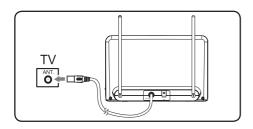
2 Connect the DC plug to the antenna and the power supply to a 120V AC outlet.
