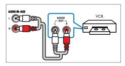
1 Using an analog cable, connect the AUX connectors on your home theater to the AUDIO OUT connectors on the TV or other device.
