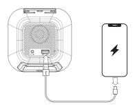
Connect the standard size end of a USB cable (not included) to the USB Port on back of the unit and connect the other end to the charging port on your device.
