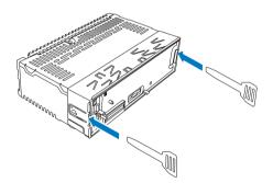
4 Install the sleeve into the dashboard and bend the tabs outward to fix the sleeve.
