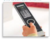
One-touch control allows you to perform multiple commands with one press of a button via a macro. A macro combines a string of pre-programmed commands under one single button. Therefore, it simply takes one button press to execute a series of functions.
