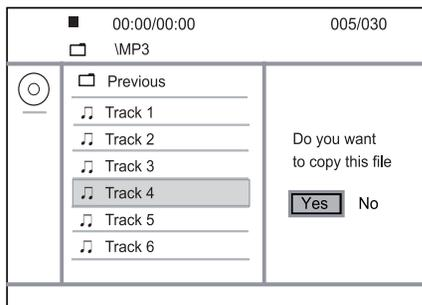
↳ Once complete, a new folder is created automatically in the USB flash drive to store all the new files.
