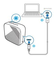
Connect the USB cable between the micro-USB socket on the speaker and a USB socket on your computer or a charger.
