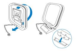
2 Connect the AM loop antenna to the AM jack on the back of the main unit.
