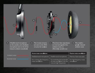
What sets the Fidelio NC1 apart from the competition is its hybrid Active Noise Cancellation (ANC) proficiency. The NC-1 uses a feed-forward and feed-backward ANC solution, which features 4 microphones implemented inside and outside the ear cans that capture noise for advanced processing. This combination ensures cancellation over a wide yet deep frequency range for optimized music enjoyment in any environment.
