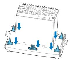
4 Attach the controller panel of the original air conditioner to the unit.
