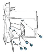
6 Slide the unit into the dashboard and fix it to the car with screws (removed from the original in-car system).
