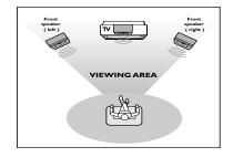
Place the front left and right speakers at equal distances from the TV set and at an angle of approximately 45 degrees from the listening position.
