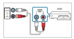
Using an analog cable, connect the AUDIO IN-AUX connectors on your SoundBar to the AUDIO OUT connectors on the TV or other device.
