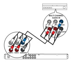
1 Connect the audio cables (not supplied) to the AUDIO OUT (FRONT L/R, REAR L/R, CENTER and SUBWOOFER) jacks on this DVD player and the audio input jacks on the device.
