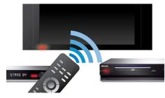
EasyLink lets you control multiple devices like DVD players, Blu-ray players, soundbar speakers, Home theatre systems and TVs etc. with one remote. It uses HDMI CEC industry-standard protocol to share functionality between devices through the HDMI cable. With one touch of a button, you can operate all your connected HDMI CEC-enabled equipment simultaneously. Functions like
