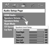
4 Use ◀ ► keys to set the volume level for each speaker (-6dB ~ +6dB) and press OK to confirm. 5 Use ▲▼ keys to highlight { Speakers Delay }, then press ▶.
