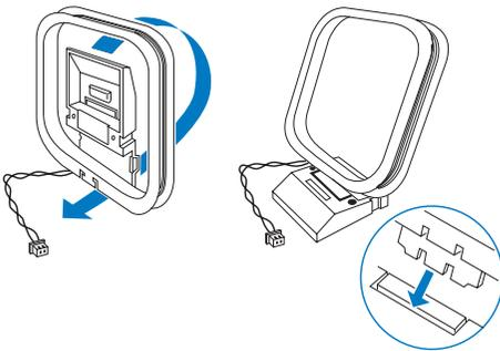
2 Connect the AM loop antenna to the **AM** jack on the back of the main unit.
