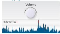
Anti-Clipping lets you play music louder and keeps it high quality, even when the battery is low. It accepts the input signals from 300mV to 1000mV and keeps your speakers safe from damage by distortion. This speaker handles anti-clipping through a dedicated audio limiter IC. This monitors the musical signal as it goes through the amplifier and keeps peaks within the
