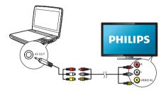
Match the color of the AV cables (the AV cable connected to TV is not supplied) with the jacks:
