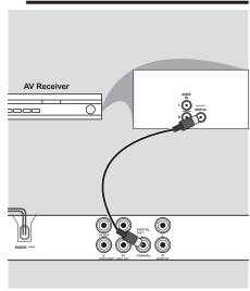
Receiver has a PCM, Dolby Digital or MPEG decoder
