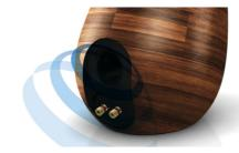
Bass-reflex acoustic load uses a bass pipe tuned to the acoustic volume of the speaker box, in order to reproduce deep bass from compact enclosures. The carefully designed profiled bass-pipe helps air flow and allows for deep and impactful bass, even at loud volumes while minimizing air turbulence that may cause distortion.
